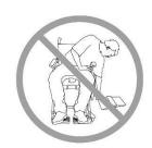
**USERS MUST NOT** position the Züm-AP/SP on a side slope as this could cause it to tip.
