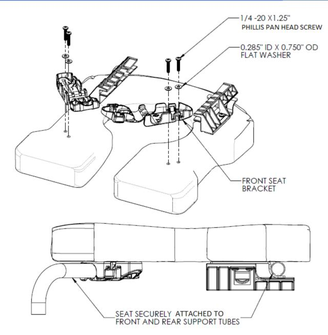
We have improved the design of our front seat brackets. Similar to the original design in its provision of stability, this design also provides improved durability and functionality.
