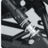
Fourfold adjustable frame suspension system which can be easily adjusted without tools.
